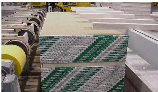
More than half of the gypsum wallboard manufactured in the United States utilizes synthetic gypsum from coal-fueled power plants.
