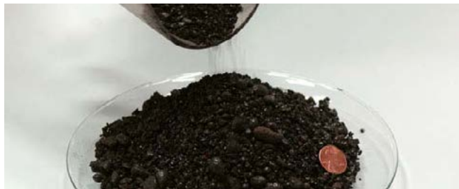
Nearly 90 percent of all boiler slag is beneficially used.
